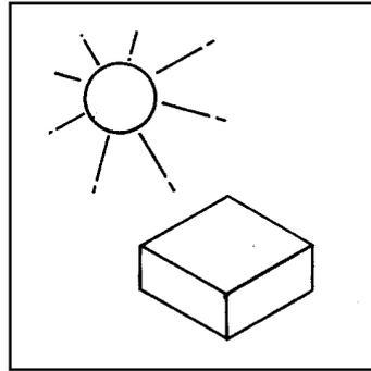
The adobe production basically consist in moulding soil prepared in a plastic state and drying it naturally on the ground. The necessary quantity of water is about one fourth of the dry earth volume.
